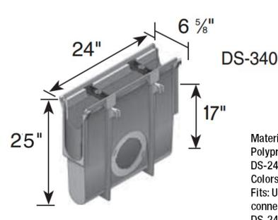
Material: DS-340: UV Protected High Density Polypropylene (HDPE) DS-240: Zinc Plated Steel Colors: Gray (DS-340), Zinc Plated Steel (DS-240) Fits: Use with NDS Universal Outlets for pipe connections.
